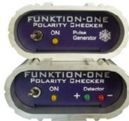
The ASPC1 is a two-part system comprising a pulse generator and a detector. The pulse generator allows you to inject a special test signal anywhere in the signal path whilst the detector microphone lets you check the resulting loudspeaker polarity acoustically. See the ASPC1 user guide for more information.
