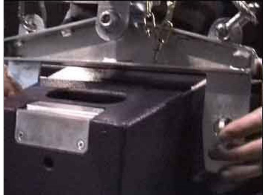
The integral toggle pins pass through holes in the CH5 column hangers.
