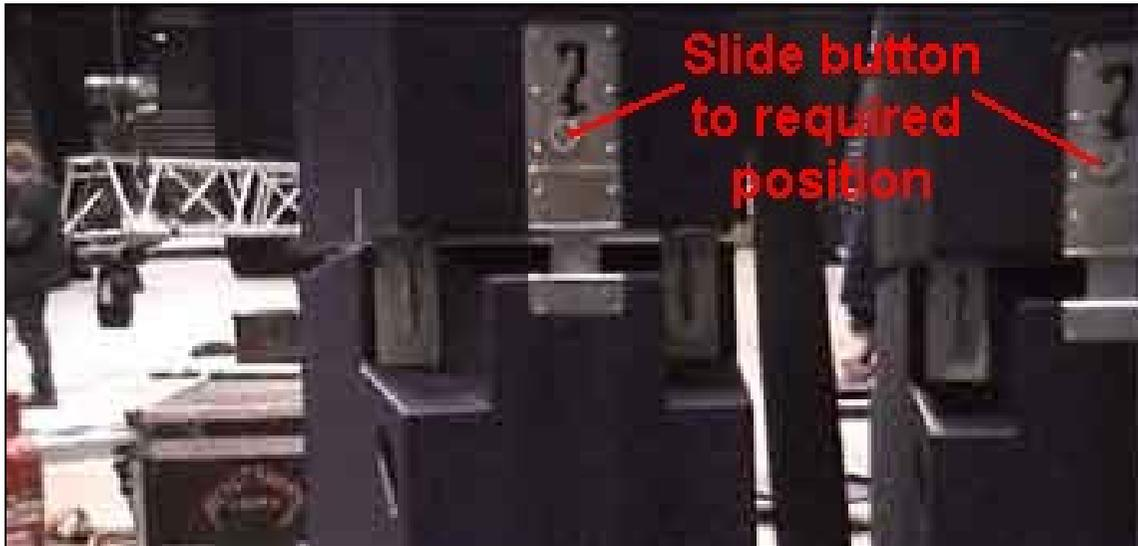
The 'Biscomatic' auto spacer must be set to achieve the required vertical splay angle between enclosures.
