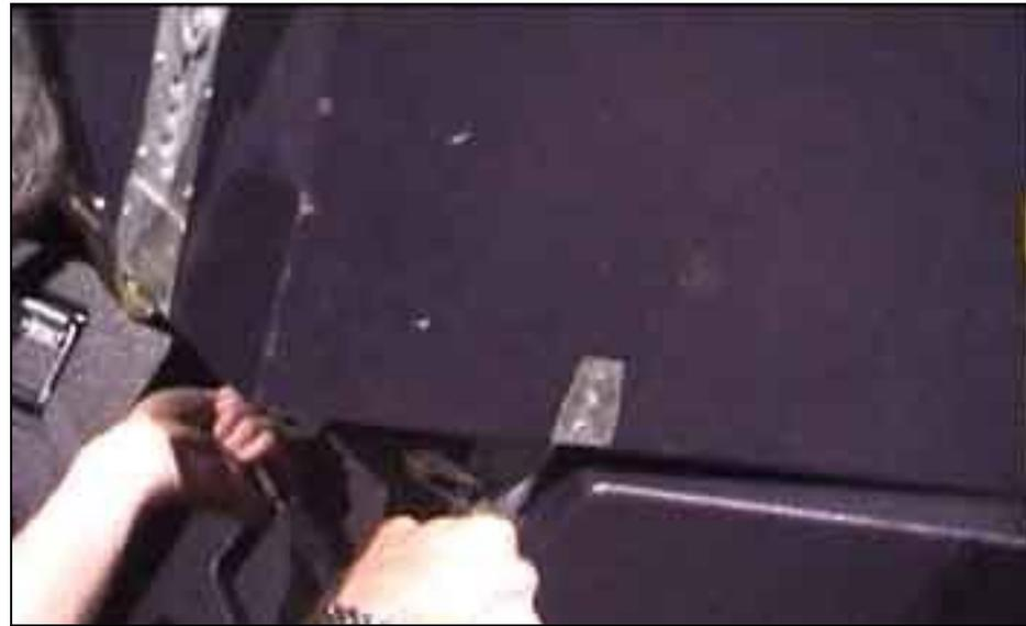
Again, sprung flying tabs are hinged out from the bottom of the cabinets above and mated with the downfills' toggle pins
